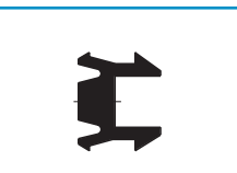
Part. 370 - Pag. S70 Sealing profile for Part.422. Improves Guide cleanliness.
